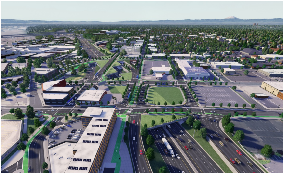
Figure 5. Broadway/Weidler/Williams and Vancouver/Hancock Highway Covers
